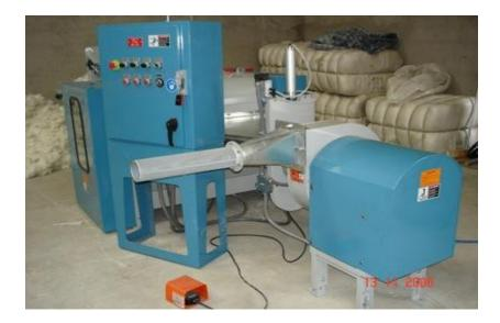
CCS offers many options such as multiple operator fiber filling stations, weigh system, timer feed controls, bar coding, variable speed motor drives, metal detection and humidification. Some custom systems are capable of producing as much as 3,000 pounds per hour. These systems generally include complete bale breakers that further reduce the labor requirement.
